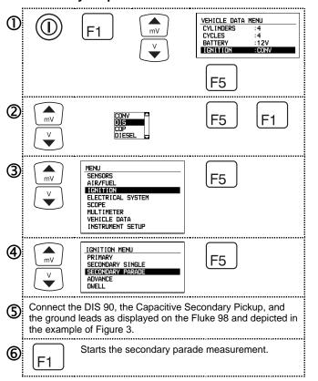
Start the engine and observe the measurement result. See an example display in Figure 5.
