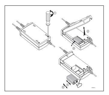
Figure 7. Replacing the Battery
